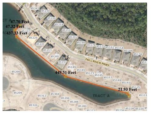
**Remove vegetation:** Remove all the vegetation down to clean soil for the area of the bank re-slope. This area is approximately 18'x1000' down one side of the shoreline that has been discussed on-site pond 14. We are estimating for 9' out of water and 9' in water for the clearing of vegetation. This may vary depending on location along the existing shoreline.
