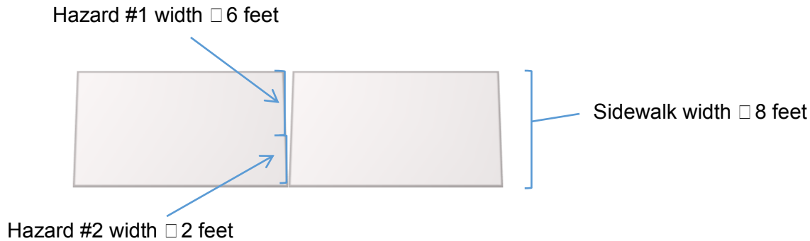
figure 1 Panels Over 6 feet Wide
